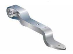
3-D trailing arms: The ingenious "three-dimensional trailing arm" (3-D) enables vehicle manufacturers to assemble air-sprung triaxle suspension systems with an LL self-steering axle onto the same frame as a rigid unit without any problems – there's no need to have a special offset frame. It goes without saying that the 3-D trailing arm offers the same functions and quality features as BPW trailing arms for rigid axles.
